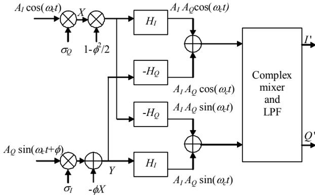
Figure 11: Amplitude and phase compensated I/Q demodulator
