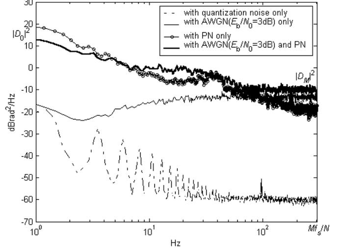
Figure 6: Decision-directed phase detector output's PSD for 4800bps BPSK with Fig. 4's oscillator PN,  $K=0.1$  and  $M=N/2$
