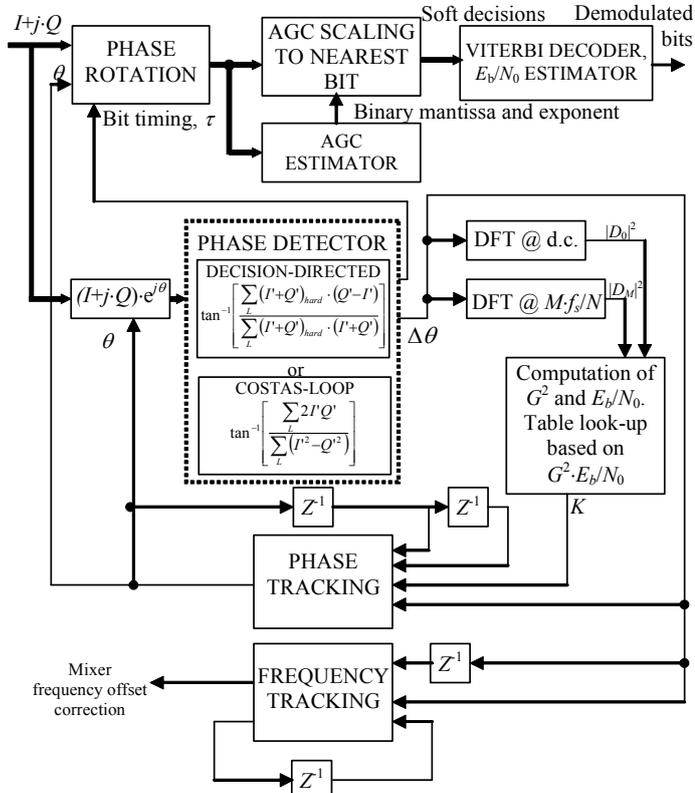
Figure 5: BPSK decision-directed block phase estimator, 2<sup>nd</sup> order phase tracker
