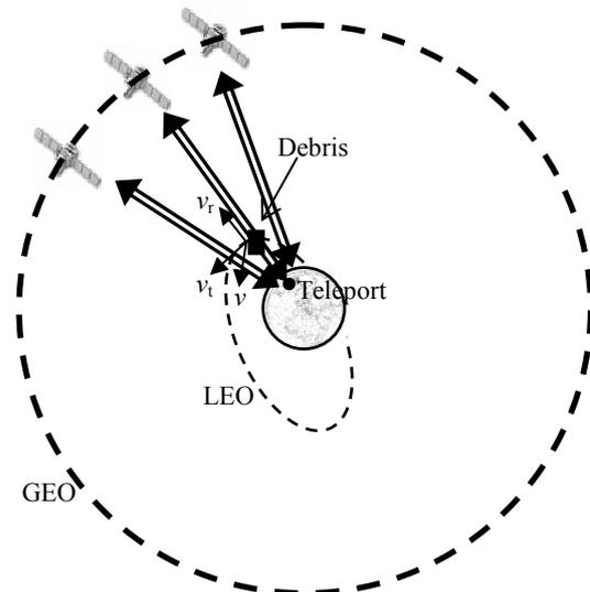
Figure 2. Antennas at each teleport pointing to different satellites
